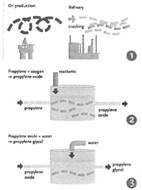
The resulting material is a mixture of mono-, di- and tri-propylene glycols that are then distilled to purify to the different grades of propylene glycol.
